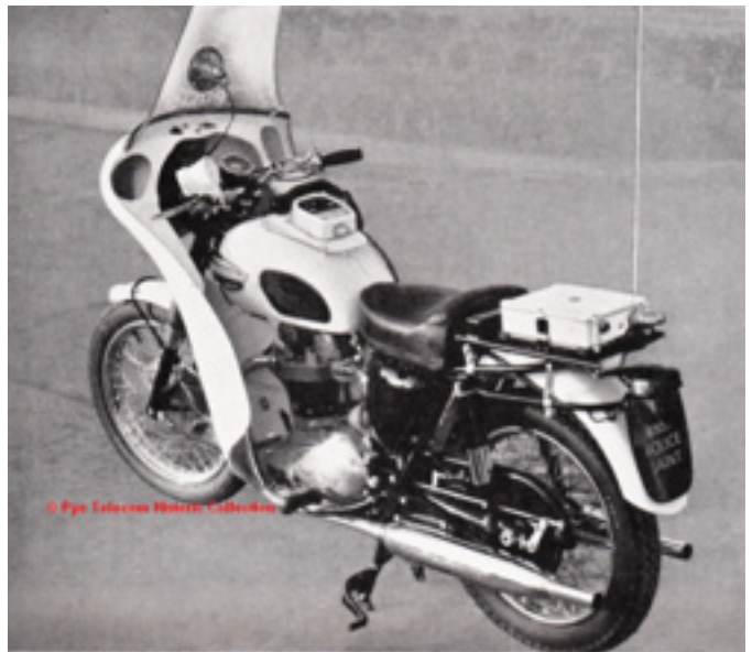
Police motor bike with installed radio set With thanks to the Pye Telecom Historic Collection
