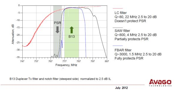
This graphically illustrates the relationship between filter performance and bandwidth and insertion loss and characterises the performance cost imposed by the proximity of Band 14 to Band 13.
