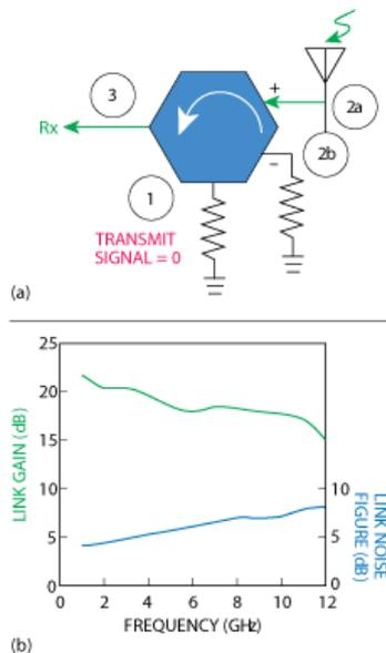
At frequencies where the impedance at the two bidirectional ports are equal, the transmit signal at Port 1 is routed to the antenna connected to port 2 and the signal received by the antenna is routed to Port 3. Port 3 is isolated from Port 1 because the portion of the transmit signal that is reflected by the antenna back into Port 2 (a) is balanced by the transmit signal reflected back into the 'balance' port 2(b) by the impedance connected to the fourth port.
