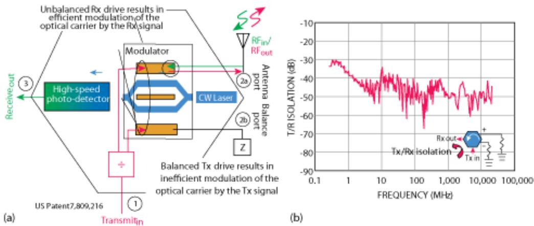
Mismatch is managed by connecting a variable impedance to an additional 'antenna balance' port which replicates antenna impedance versus frequency.
