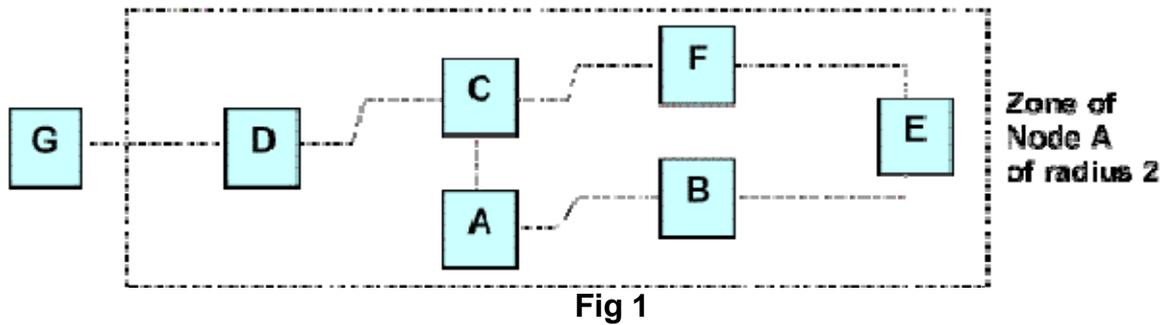
The box defines a zone in which the minimum distance from any device to any other device is never more than 2 hops. Nodes B through F are within the routing zone of A, node G is outside A's routing zone.
