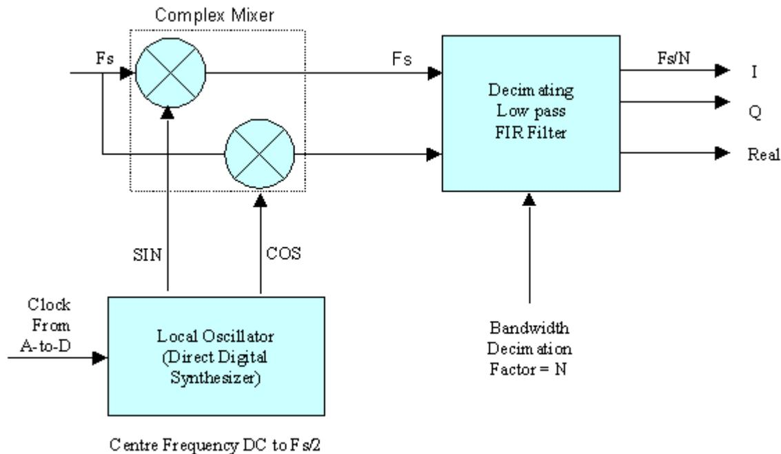
The samples are passed to a pair of digital mixers or multipliers where they are multiplied by the output from a digital oscillator. The digital oscillator generates precise [eg 32 bits precision (or greater)] digital value samples of both a sine and cosine wave. As the oscillator is clocked with the same clock ( $F_s$ ) as the ADC the sine/cosine samples are generated at the same time as the A to D sample conversion takes place.
