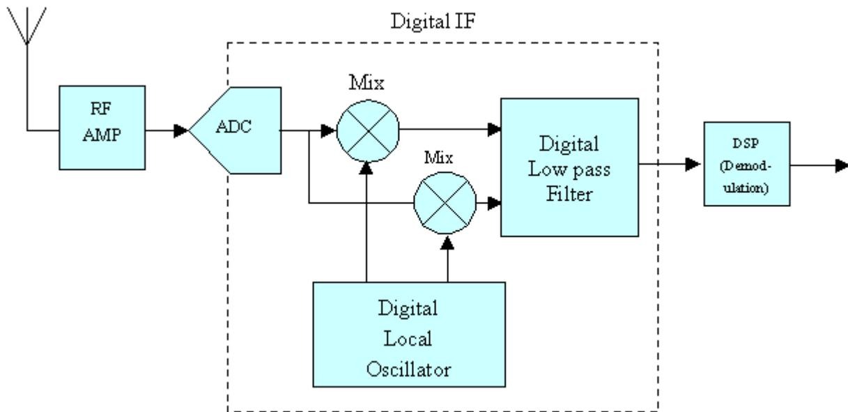
So far these topics have addressed the signal processing parameters principally in terms of ADC and demodulator performance. However, if improved performance, ie sensitivity, selectivity, cost, is to be achieved, the RF and IF processing before analogue to digital conversion must be considered in detail. Equally, the processing after signal conversion must be considered in detail if 'best performance' is to be obtained.
