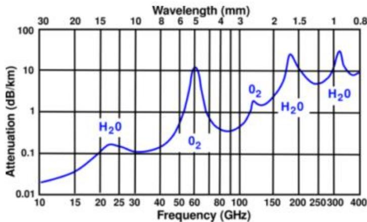
The transmission windows for longer links (up to 60 km) include the 5 G-E band options at 72-77 GHz (4.16-3.89 mm), 81-86 GHz (3.7-3.48mm) and 92-95 GHz (3.25mm-3.15mm) presently used for lightly licensed fixed point to point backhaul and proposed for use for military communication based on rapidly deployable sub space systems to provide high data rate wide area coverage.
